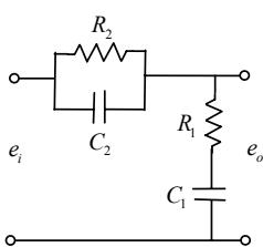
$$\begin{aligned} \frac{E_0(s)}{E_1(s)} &= \frac{R_1 + \frac{1}{C_1 s}}{\frac{1}{(1/R_2 + C_2 s)} + R_1 + \frac{1}{C_1 s}} \\ &= \frac{(R_1 C_1 s + 1)(R_2 C_2 s + 1)}{(R_1 C_1 s + 1)(R_2 C_2 s + 1) + R_2 C_1 s} \end{aligned}$$
