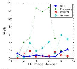
(a) Comparison of the MSE between motion parameters estimated by various registration methods and the known parameters.
