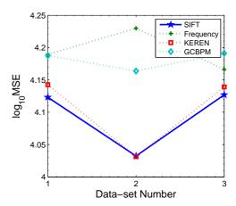
(b) Quantitative comparison of the SR output with different registration methods for each data set. MSE is between produced HR images and the original HR images.
