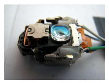
Step 3: Solder wires to the lens head
