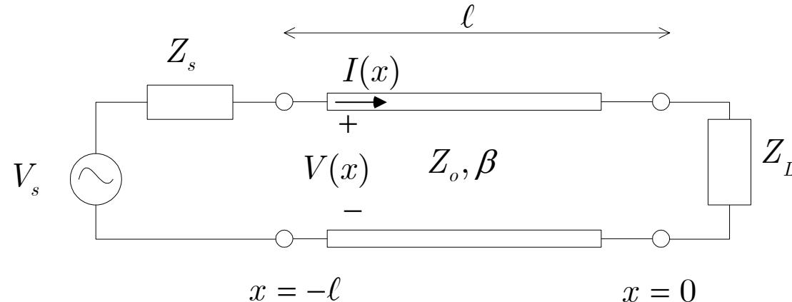
Tx-line excited by voltage source  $V_s$  operating at frequency  $\omega$  and internal impedance  $Z_s$ . The line is terminated by the load  $Z_g$ . The source will excite the line voltage. The load will result in reflection of the voltage and current waves, leading to standing waves on the line in the steady state condition.
