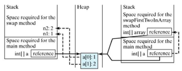
Invoke swap(int n1, int n2). The arrays are The primitive type values in a[0] and a[1] are passed to the swap method.
