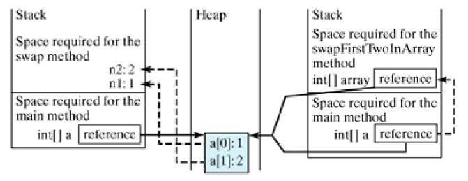
Invoke swap(int n1, int n2). The arrays are Invoke swapFirstTwoInArray(int[] The primitive type values in stored in a array). The reference value in a is passed a[0] and a[1] are passed to the heap. to the swapFirstTwoInArray method. swap method.
